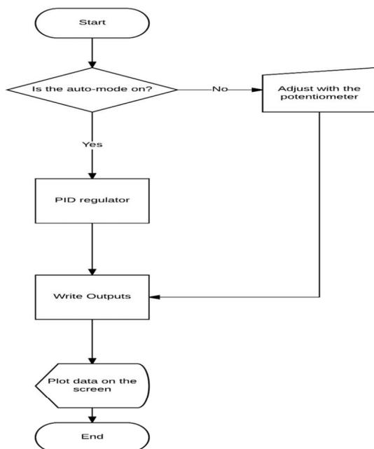
The Arduino IDE was used to code the program for the system, and the sketch was divided in three main parts: the data acquisition, the regulation process and the screen menu navigation.
