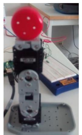
Robot arm of 2DOF (2 degrees of freedom) with a couple of stepper motors and 2 bars
